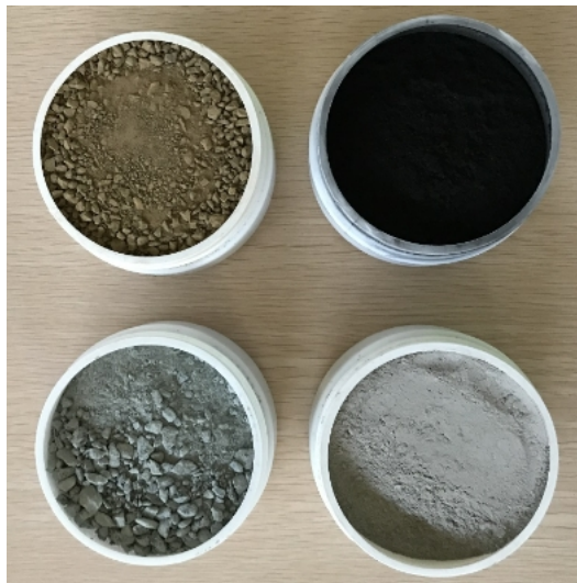
Figure 4. Samples used in factory testing program loaded into standard 100 mm diameter containers; coarse chips (left) and dried process pulps (right). Lids have been removed to illustrate the contents.
