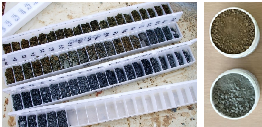
Figure 7. (Left) Chip-trays created by RC drilling. (Right) PhotonAssay™ jar of sampled core material after crushing to a top-size of approximately 2-3 mm. (Chip-trays image credit: MinAnalytical Laboratory Services.)
