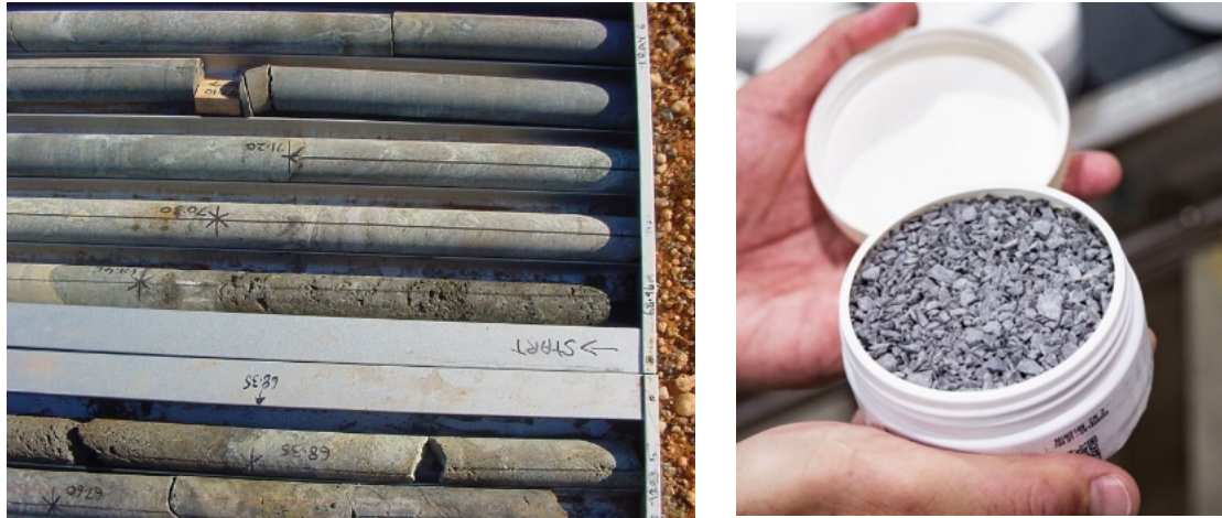
Figure 6. (Left) Dried drill-core samples in trays. (Right) PhotonAssay™ jar of sampled core material after crushing to a top-size of approximately 2-3 mm. (Core image credit: MinAnalytical Laboratory Services.)
