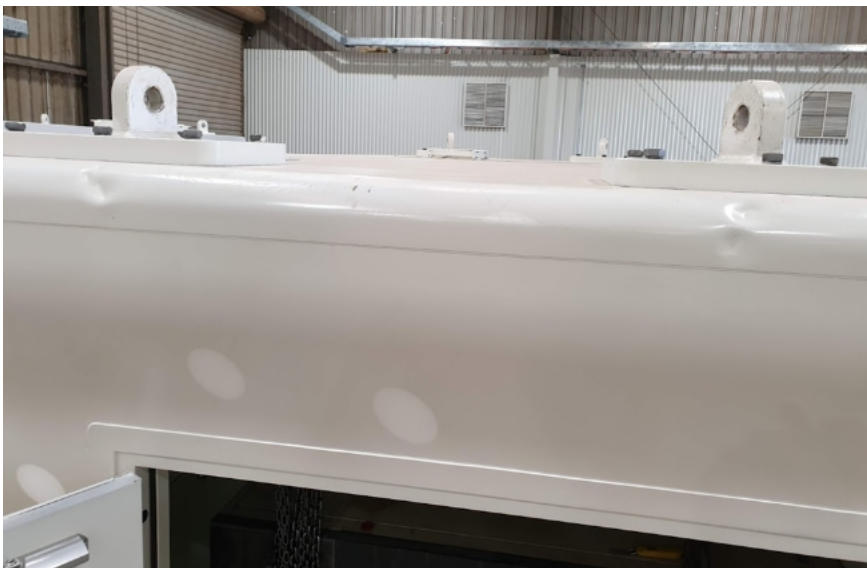
Figure 7 shows damage that will occur to the cabins if not protected from the chains.
