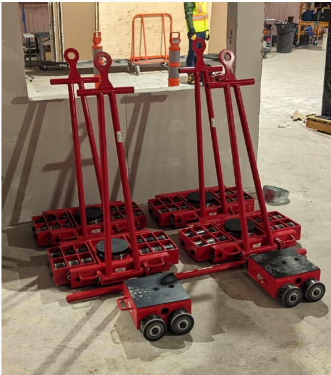
Figure 14 shows the Trolleys/Tanks that the cabins are unloaded onto.
