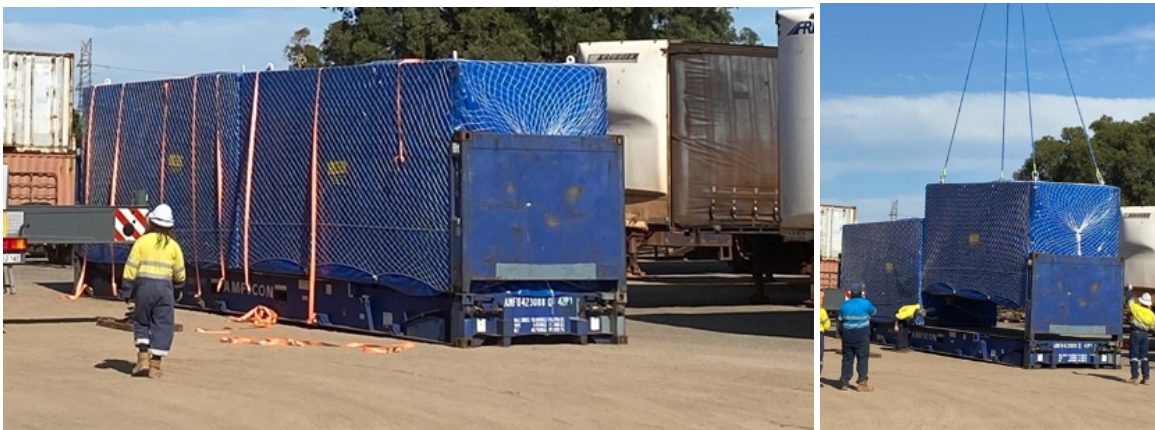
a) Flat rack with 2 lighter cabins
