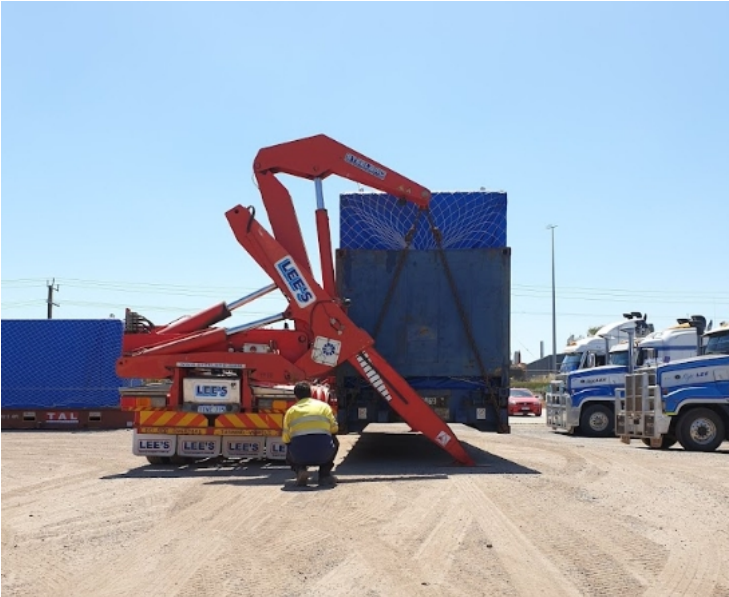
Figure 4 shows a 'side loader' unloading a flat rack container - this is not possible with the cabins.
