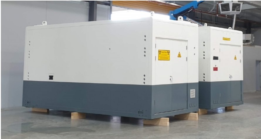
Figure 24 Cabins resting on timber blocks.
