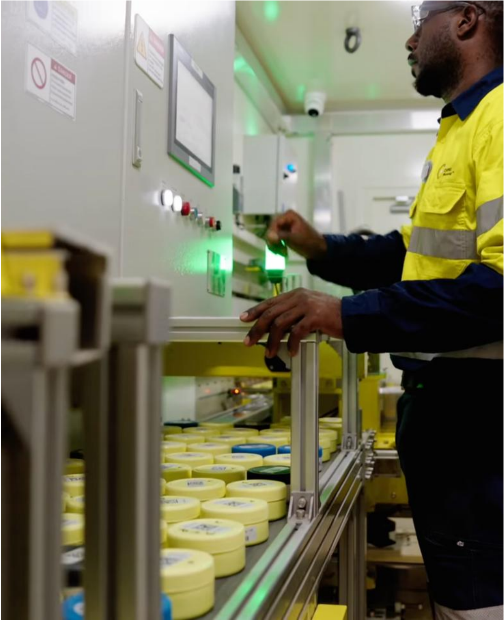
PhotonAssay™ Unit & Chrysos Maintenance Engineer
